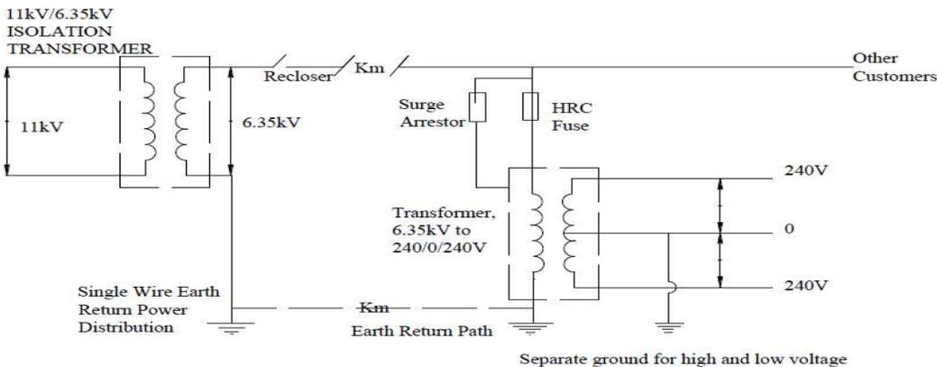
Fig. 2. SWER model showing isolation and distribution transformers, and earth return path
