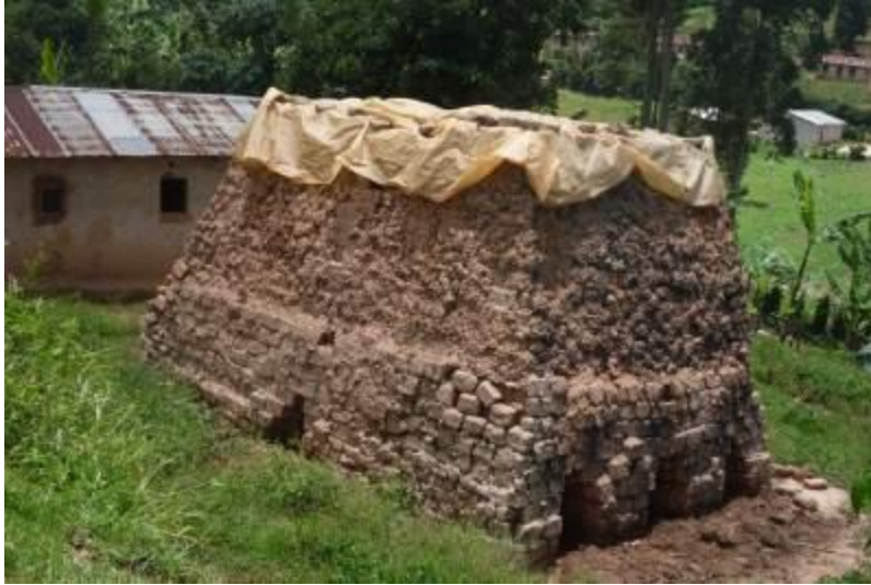
Figure 93 Modern brick kiln made of hand made bricks and an outside layer of mud. Wood in the hollow chamber bakes the bricks from the inside. Straw and plastic protects bricks from rain erosion. Usually found around clay beds and construction sites.
