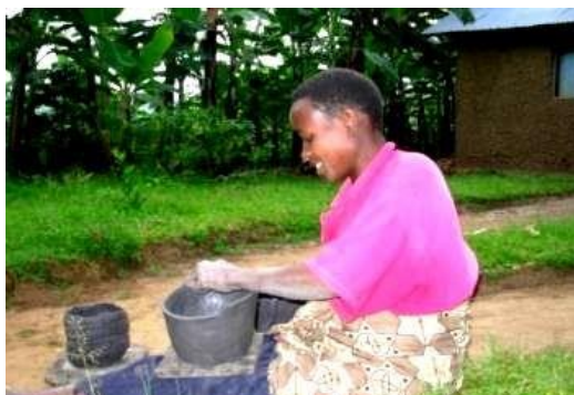
Fig. 3. Making clay stoves using coils
