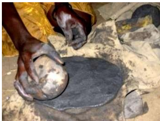
Fig. 4. Making a slab using a pebble
