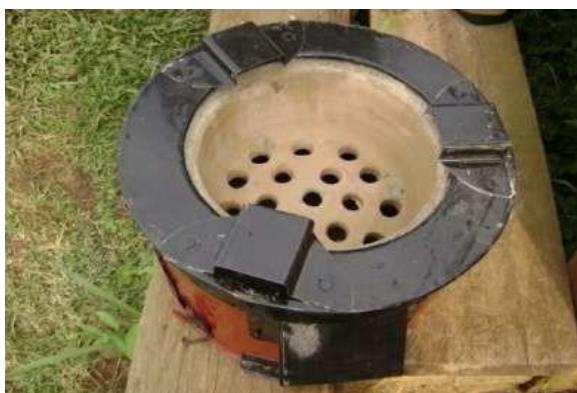
Fig. 15. Energy saving stove with a ceramic insert
