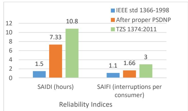
Fig. 3. Reliability indices between distribution system and set standards
