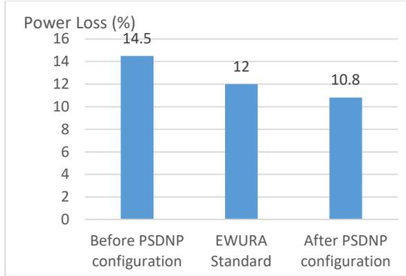
Fig. 4. Power distribution losses before and after PSDNP
