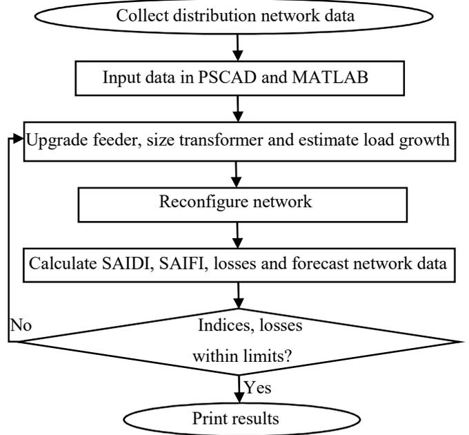
Fig. 1. Flowchart for proposed planning scheme
