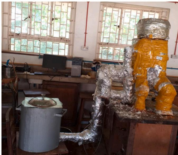
Fig. 3. Constructed experimental set up system showing an insulated TES tank, insulated charging unit, insulated connecting pipes and the cooking unit.
