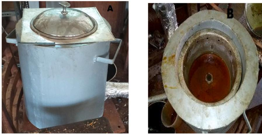
Fig. 5. Images of the cooking unit (A): with the cooking pan inserted and (B) with the cooking pan removed.
