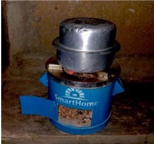
**Figure 6.** Smart home stove insulated with metal.
