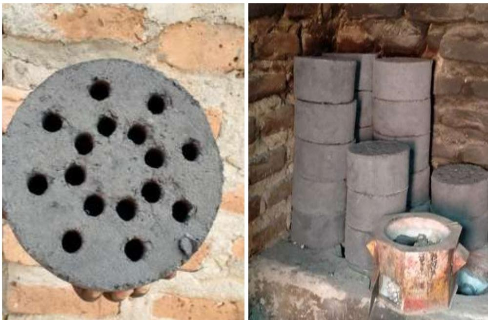
**Figure 9.** Beehive briquette piled in the kitchen ready for cooking.
